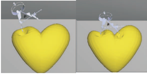
Fig. 12. Two contact regions between a rigid compass and a deformable heart: (left) one contact region (right) two contact regions
