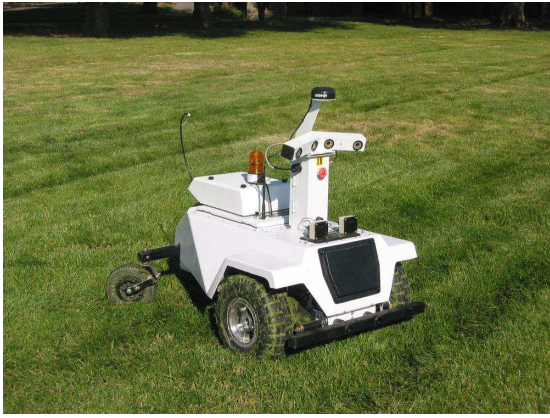
Fig. 1. Ground rover platform instrumented with inexpensive IMU and GPS. This robot is commercially provided to contractors in the DARPA LAGR program.
