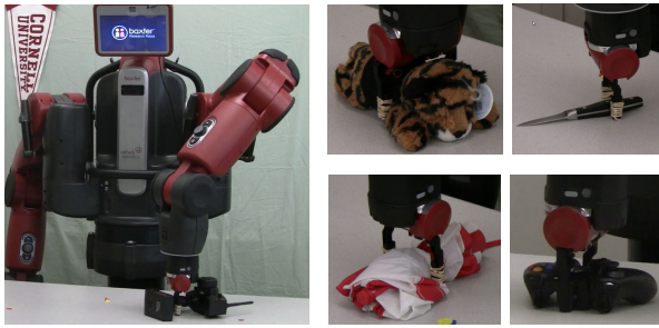
Fig. 10: Baxter grasping objects. Our Baxter robot grasping objects using our algorithm.
