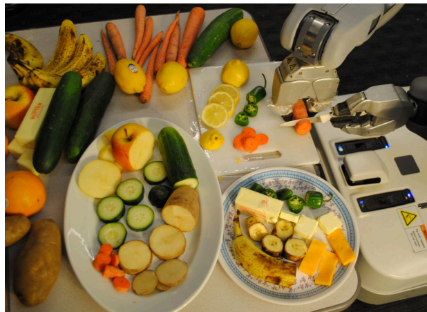
Fig. 1: Cutting food: Our PR2 robot uses our algorithms to perform complex, precise food-cutting operations. Given the large variety of material properties, it is challenging to design appropriate controllers.
