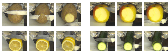
Fig. 9: Cutting food: Time-series of our PR2 robot using our DeepMPC controller to cut several of the food items in our dataset.
