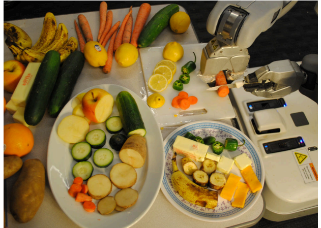
Fig. 1: Cutting food: Our PR2 robot uses our algorithms to perform complex, precise food-cutting operations. Given the large variety of material properties, it is challenging to design appropriate controllers.
