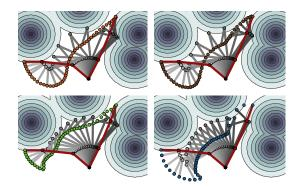
Fig. 3: Robot 3DoF. Trajectory after 10 iterations: top-left: Gaussian RBF kernel, top-right: B-splines kernel, bottom-left: Laplacian RBF kernel, bottom-right: waypoints.
