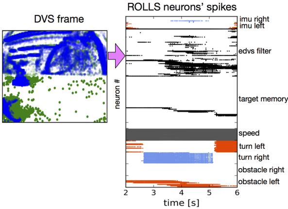
Fig. 9: Robot approaching a target robot while avoiding an obstacle on the way. **Top:** Image of DVS events accumulated over 1.5s marked by the gray area in the bottom plot. **Bottom:** Activity on the ROLLS for the labeled neural populations.
