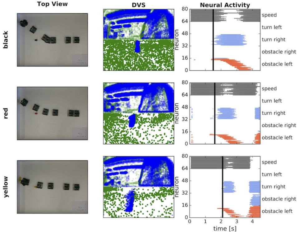
Fig. 6: Response of the robot to different obstacle colors. **Left:** Overlays of the overhead camera images with fixed time intervals to indicate the speed. **Center:** Image of DVS events accumulated over 1.5s up to the start of the turn, indicated by the black vertical line in the neural activity plot. **Right:** Neural activity on the ROLLS for the neural populations that control the avoidance maneuver.
