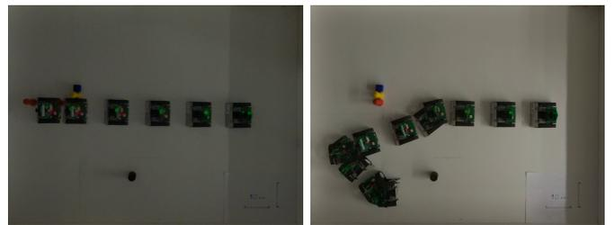
Fig. 7: Overlaid images of the robot trajectory in the arena at different lighting conditions. **Left:** Dark, robot fails to perceive an obstacle. **Right:** Lighter, but still less light than at day time, the robot avoids obstacles successfully.
