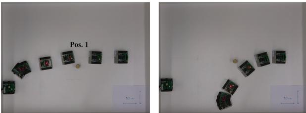
(a) Successful target acquisition and obstacle avoidance. (b) Target is lost from sight after avoiding an obstacle.
