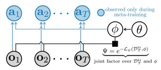
Fig. 3. Graphical model underlying our approach. During meta-training, both the observations  $\mathbf{o}_t$  and the actions  $\mathbf{a}_t$  are observed, and our method learns  $\theta$  and  $\Psi$ . During meta-testing, only the observations are available, from which our method combines with the learned prior  $\theta$  and factor  $\Psi$  to infer the task-specific policy parameters  $\phi$ .
