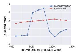
Fig. 7: Performance comparison of controllers that are trained with (red) and without (blue) randomization and tested with different body inertia.
