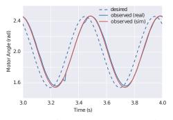
Fig. 4: Comparison of the simulated motor trajectory (red) with the ground truth (blue).
