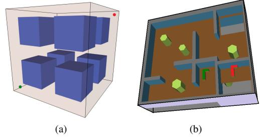
Fig. 4. Two of the scenarios used in the experiments. (a)  $dD$  Hypercube with  $2^d$  hypercubical obstacles, and (b) 3D Cubicles. Start and target configurations for a robot are depicted in green and red, respectively. Scenario (b) is provided with the OMPL distribution.
