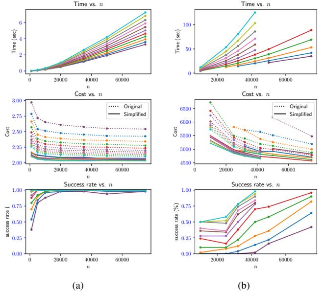
Fig. 6. (a) FMT\* for a point robot in the 4D hypercube with obstacles scenario (Figure 4a) (b) FMT\* for two rigid-body robots moving in OMPL’s Cubicles scenario (Figure 4b). Both the average original cost and the average cost after simplification are presented for each radius. There is a difference in cost between the various radii (dashed lines), that diminishes after simplifying the resulting paths (solid lines).
