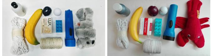
Fig. 7. Left: The objects used to reproduce the dynamic grasping in clutter experiment of [32]. Right: The test objects used by [32]. We have attempted to recreate the object set as closely as possible.
