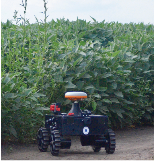
Fig. 1. The ultra-compact 3D printed field robot, termed TerraSentia, in soybean breeding plots in Energy Farm, Urbana, IL, USA.
