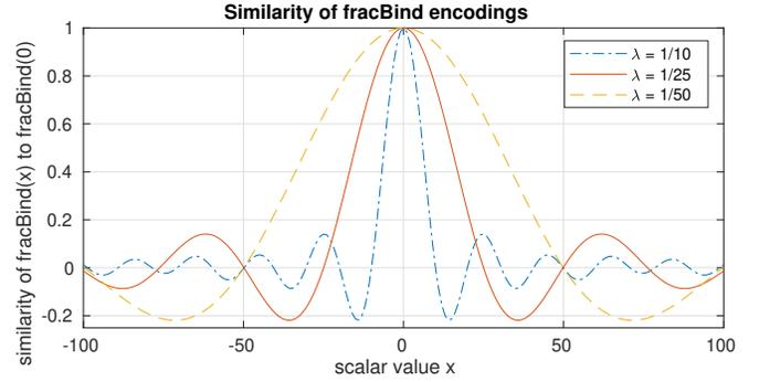
Fig. 2. Encoding similar scalar values with fractional binding results in high-dimensional vectors with high similarity. A scaling parameter  $\lambda$  can be used to influence the decay of the vector similarities. This resembles the sinc() function, the visible oscillation is a result of the periodic behavior of exponentiation in the complex domain, see [34] for more details.
