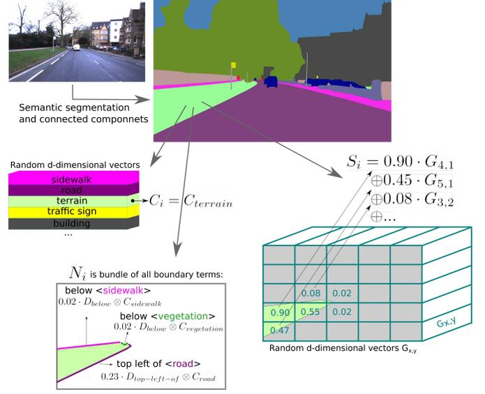
Fig. 3. Illustration of the spatial semantic information part of an image entity  $e_i$  consisting of class vector  $C_i$ , neighborhood encoding  $N_i$ , and shape/location encoding  $S_i$ . Together with the appearance encoding  $A_i$ , these vectors are the basis for the proposed vector semantic representation (VSR).
