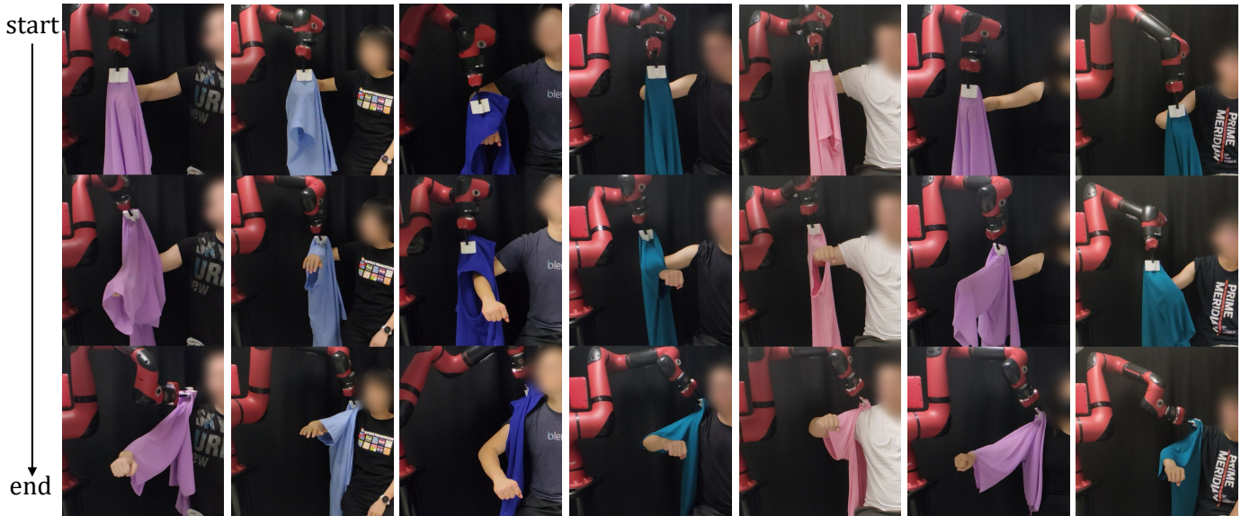
Fig. 1: We develop a robot-assisted dressing system based on a single learned policy that is able to dress different people with diverse poses and garments. Each column shows snapshots from a trajectory of our policy. We learn the dressing policy using reinforcement learning with point cloud observations to generalize to diverse garments. We use policy distillation to combine multiple policies that each work for a small range of arm poses into a single policy that works for a large variety of arm poses.
