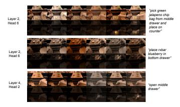
Fig. 13: In this figure we show the attention map of the RT-1 policy. Different layers and heads generally focus on different part of the image. Most commonly, they focus on the parts of the scene with the richest interaction affordances, such as graspable objets. For example, Layer 2 Head 6 focuses on the jalapeno chips and pepsi can in grasping tasks; and Layer 4 Head 2 focuses on the drawer in drawer opening tasks.
