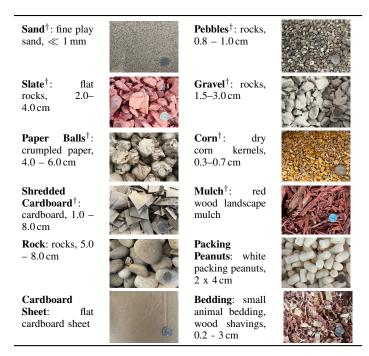
TABLE I: Materials used in each terrain, with approximate grain sizes where applicable. Images show U.S. quarter coin for scale. Training set denoted with †; testing set consists of all materials and novel material combinations.
