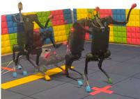
Fig. 1: Agile skills learned with our proposed method enable the A1 robot to jump repeatedly (left) and walk to a goal location on its hind legs (right).
