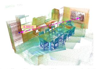
Fig. 5: **3D** spatial reasoning abilities: A key benefit of lifting foundation features to 3D is the ability to reason about spatial attributes. For example, the query "how far is the refrigerator from the television". gets parsed by our LLM-parser into the 3DSC howfar (refrigerator, television). The centroid of the point set returned by the query term refrigerator and television are shown as blue circles, and the estimated distance between them (6.303 metres) as a straight line.
