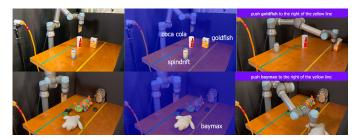
Fig. 8: Real-world **tabletop rearrangement** experiments. The robot is provided with rearrangment goals involving novel objects. (*Top row*) push goldfish to the right of the yellow line, where goldfish refers to the brandname of the pack of Cheddar snack. (*Bottom row*) push baymax to the right of the yellow line, where baymax refers to the plush toy depicting the famous Disney character.
