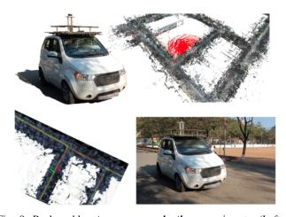
Fig. 9: Real-world **autonomous navigation** experiments. (Left to right; top to bottom) Autonomous drive-by-wire platform deployed; pointcloud map of the environment with the response to the openset text-query "football field" (shown in red); path found to the football field (shown in red); car successfully navigates to the destination autonomously. See our webpage for more results.
