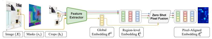
Fig. 2: ConceptFusion constructs **pixel-aligned features f**<sup>P</sup> by: processing input images to generate generic (class-agnostic) object masks (regions)  $r_i$ , computing a bounding box for each region and extracting a local feature vector  $\mathbf{f}_i^L$ , computing a global feature  $\mathbf{f}^G$  for the input image as a whole, and fusing the region-specific features with global features as illustrated in Fig. 3 and described in Sec. IV-A.
