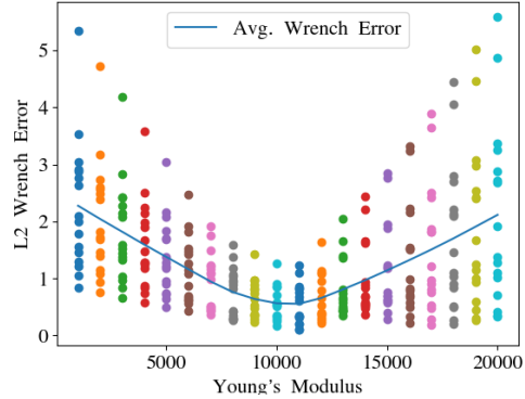
Fig. 5. We perform system identification to match simulated material properties to our real object setup. 16 real setup presses are recreated in simulation and the simulated wrench is compared to that registered in the real world. Points indicate individual simulation trial comparisons to the real world data, colored for visual clarity by the used Young’s Modulus. We found the optimal Young’s Modulus to be E = 1.1e4 Pa.
