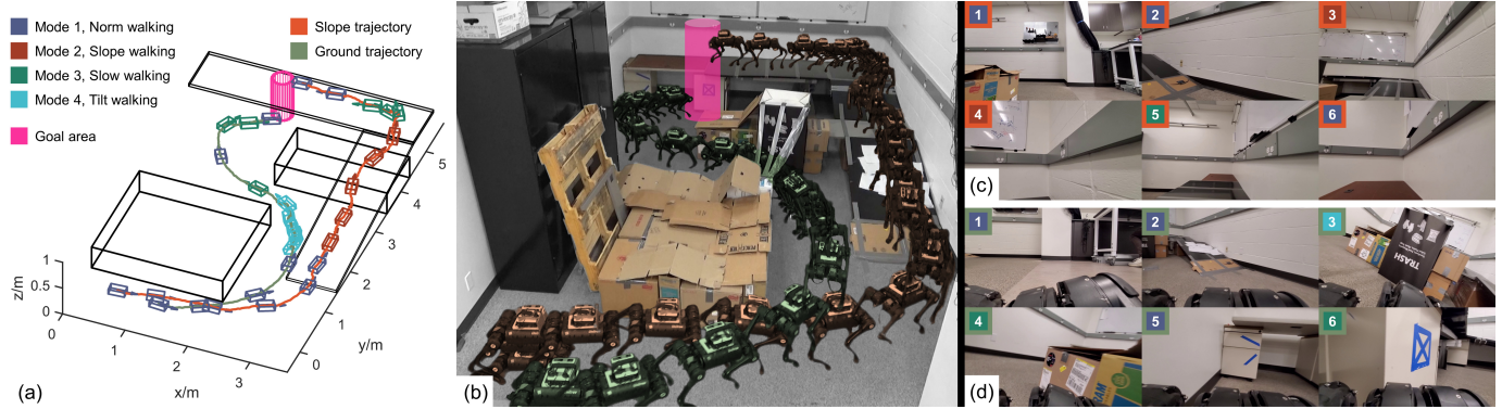
Fig. 1: We propose a generalized Hamilton-Jacobi (HJ) reachability framework to compute Backward Reachable Tubes (BRT) and safe controllers for hybrid dynamical systems with nonlinear dynamics and discrete transitions. Here, we apply the proposed framework for optimal mode planning for a quadruped robot that switches between different walking gaits (modeled as discrete modes in the hybrid system) in order to reach its goal safely (i.e., without colliding with any obstacles on the way). We compute the BRT of the robot and obtain the optimal continuous control and mode sequence from the BRT. We show the corresponding quadruped trajectories in (a). The quadruped safely navigates through the slope or narrow ground obstacles to reach the goal area (pink cylinder). The goal area is independent of the z position, so the robot can reach it via slope or ground route. Different colors along the robot trajectory correspond to different walking modes that the robot autonomously chooses to avoid collision while navigating as quickly as possible to the goal. (b) Overlaid trajectories in the real-world obstacle setup. (c, d) First-person view along the slope route (c) and the ground route (d). Videos of the experiments and source materials can be found on the project website javierborquez.github.io/HybridReachability .
