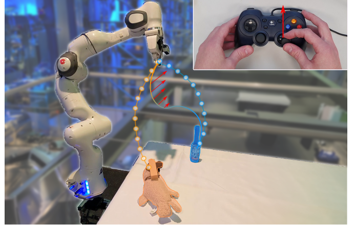
Fig. 1: A motivating application for this work is obstacle grasping with unknown task hierarchy. The robot possesses motion policies for handling both objects but initially prioritizes the orange one for pickup. However, the human operator envisions a different order and issues corrective commands via a gamepad to convey their desired direction of motion. The task is dynamically adapted to pick up the blue object instead.
