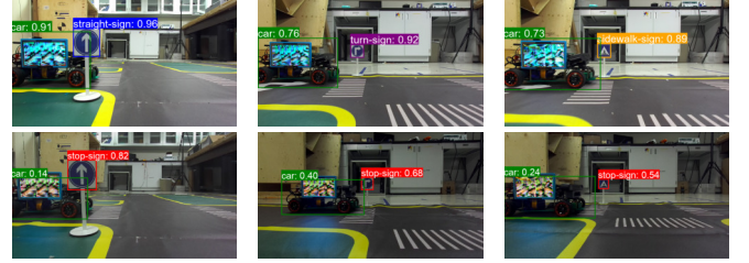
Fig. 11: Illustration of adversarial patch effectiveness without SIT-Net. The top row depicts real-world implementation results, and the bottom row shows simulation results. The columns, from left to right, represent attacks on “Go-straight”, “Turn”, and “Pedestrian” signs. This visual comparison clearly shows that the simulation without SIT-Net fails to replicate the real-world effectiveness of the patches, emphasizing the importance of SIT-Net in realistic adversarial training.
