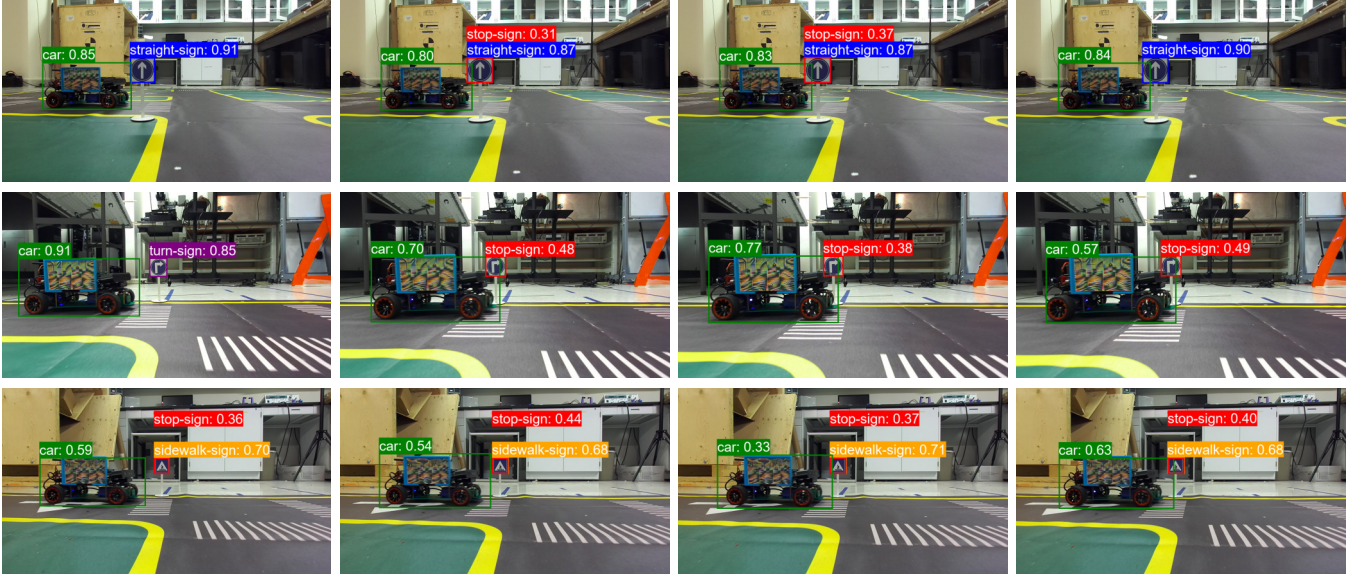
Fig. 17: Sequential frames showing the performance of adversarial printed patch attacks. The frames depict that the confidence levels of the misclassified “Stop-sign” remain below the critical threshold of 0.5 , indicating the ineffectiveness of these patches in real-world conditions.
