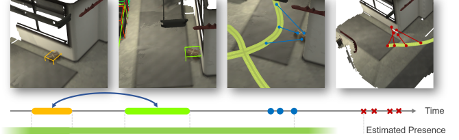
Fig. 6: Reconciliation. An object is visited twice, resulting in two fragments (orange and green). Fragments are associated via global optimization (blue arrow). Even without semantic detection, geometric verification provides evidence of presence or absence. We estimate the object must have disappeared in between the last presence and first absence observation.
