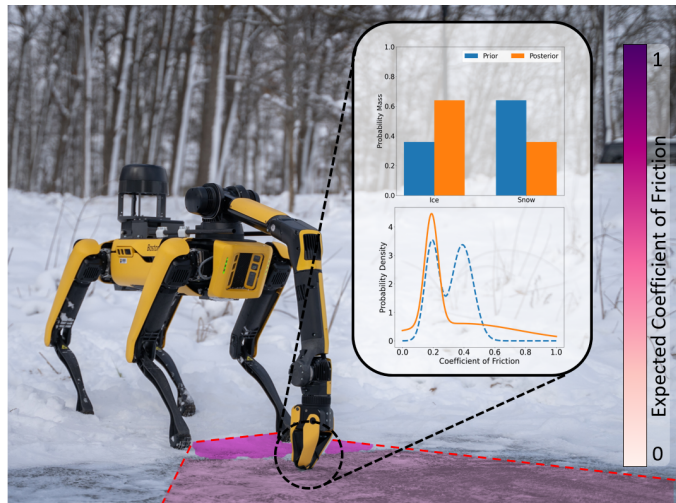
Fig. 1: The method proposed in this paper jointly estimates semantic classifications and physical properties by combining visual and tactile data into a single semantic mapping framework. RGB-D images are used to build a metric-semantic map that iteratively estimates semantic labels. A property measurement is taken which in turn updates both the semantic class predictions and physical property estimates. In the depicted example, the robot is unsure if the terrain in front of it is snow or ice from vision measurements alone (prior estimates) which dramatically affects the coefficient of friction and the associated gait that can be applied to safely traverse the terrain. The robot uses a tactile sensor attached to its manipulator to update its coefficient of friction estimation (posterior estimates), which then enables it to change gaits to cross the ice safely.
