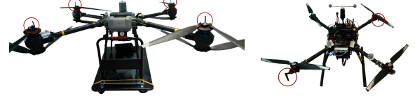
Fig. 13: Illustration of the used hardware platforms. The mothership (left) and parasite (right) used in our experiment. The dark red circles highlights the equipped UWB sensors.
