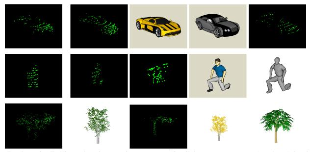
Fig. 5. Exemplar matches. The leftmost column shows example segments extracted from 3D laser scans: car, person, tree (top to bottom). Second to last columns show exemplars with distance below threshold, closer exemplars are further to the left.
