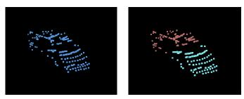
Fig. 2. (left) Laser points of a car extracted from a 3D scan. (right) Segmentation via mean-shift. The soup of segments additionally contains a merged version of these segments.
