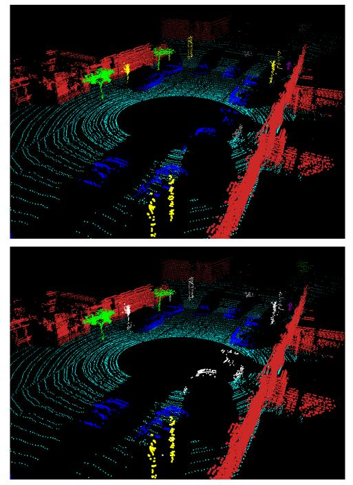
Fig. 6. (top) Ground truth classification for part of a 3D laser scan. Colors indicate ground plane (cyan) and object types (green: tree, blue: car, yellow: street sign, purple: person, red: building, grey: other, white: not classified). (bottom) Classification achieved by our approach. As can be seen, most of the objects are classified correctly. The street signs in the back and the car near the center are not labeled since they are not close enough to any exemplar.
