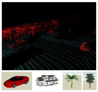
Fig. 1. (Upper row) Part of a 3D laser scan taken in an urban environment (ground plane points shown in cyan). The scan contains multiple cars, a person, and trees and buildings in the background. (lower row) Example models from Google's 3D Warehouse.
