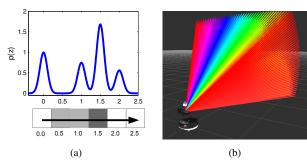
Fig. 3: Beam based measurement model: (a) 1 beam, the cells it intersects at various distances, and the resulting distribution over measurements when  $z_{\rm min}=0.5$  and  $z_{\rm max}=2$ . Darker cells have a higher probability of being occupied. (b) Raycasts for multiple beams. Obtained from Charrow et al. [5].
