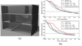
(a) Stairwell with walls removed (b) Map entropy over time using random (top) and lattice (bottom) local motions with and without trajectory optimization
