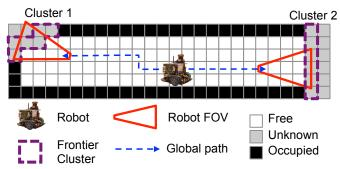
Fig. 5: **Global Planning**: Generate global plans by 1) clustering frontier voxels and 2) planning paths to places that can view them. When a robot can view a cluster from many places, we pick the one that can be reached the fastest.
