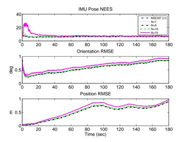
Fig. 2. Simulation results: the position and orientation RMSE, as well as the IMU-pose NEES over time. Plots are averages over 100 Monte-Carlo trials. The compared methods are the MSCKF 2.0 (blue dash-dotted line), and the DEEP-MSCKF with N = 1 (red dotted line), N = 5 (black dash-dotted line), N = 10 (green dashed line), and N = 15 (magenta solid line).
