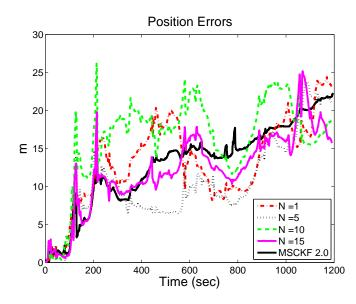
Fig. 5. Real-world experiment: position errors of the MSCKF 2.0 and the DEEP-MSCKF for increasing N.
