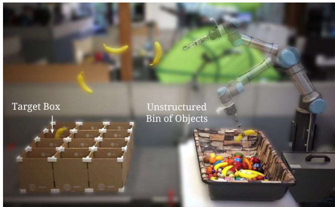
Fig. 1. TossingBot learns to grasp arbitrary objects from an unstructured bin and to throw them into target boxes located outside its maximum kinematic reach range. The aerial trajectory of different objects are controlled by jointly optimizing grasping policies and throwing release velocities.
