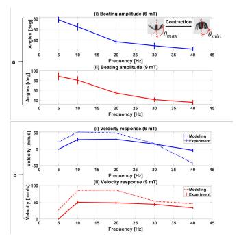
Figure 5. The influence of actuation frequencies on the robot's kinematics and swimming performance. The velocities and kinamtics at different actuation frequencies are shown in Video part 1. (a) The variation of the beating amplitude with the increasing actuation frequency. (b) The variation of the swimming speed with the increasing actuation frequency. The error bars represent the standard deviation.
