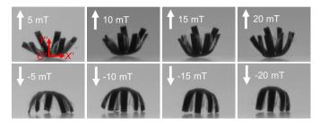
Figure 2. Deformation of the robot under constant B fields with different magnitudes. The body-attached frame is plotted in red.
