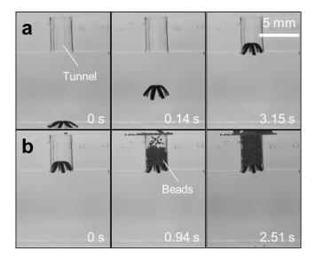
Figure 7. Tube/channel clogging (embolization) demonstration: (a) The robot swims from the tank bottom and docks at the orifice of the tube. (b) The beads pumped from the top are blocked within the tube. See Video part 2 for the details.
