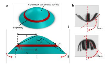
Figure 3. Illustration of the simplified dynamic model. (a) Schematic illustration: (i) The thrust force is estimated by integrating the drag force acting on the stripe ring with infinitesimal width (dl); (ii) The geometry parameters used in the simplified model. (b) The beating angles achieved when the robot lappets deform to extreme positions.
