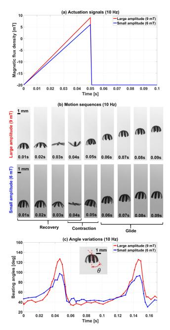
Figure 4. Actuation signals and kinematics of the robot at actuation frequency of 10 Hz. (a) Large and small actuation signals. (b) Motion sequences under these two actuation signals. A complete cycle includes three phases: recovery phase, contraction phase, and glide phase. The kinamtics at different actuation signals are shown in Video part 1. (c) Variations of the beating angles of two actuation signals within two cycles.
