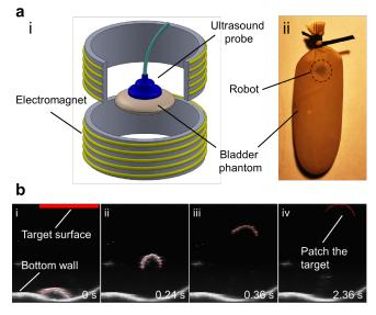
Figure 8. Demonstration of patching a target surface inside a bladder model by the robot, guided by ultrasound imaging: (a) The experiment setup: (i) The coil system; (ii) The bladder phantom. (b) Patching the target surface by the robot while guiding it under ultrasound imaging. The target surface is marked with a red thick line. The robot body is marked with thin red curves. See Video part 2 for the details.
