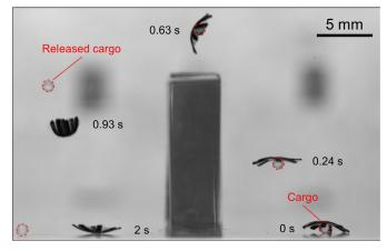
Figure 6. Cargo transport demonstration of the robot: The video snapshots of the robot and the bead are overlayed in the same video image. The red dashed circles indicate the positions of the bead being trapped and transported by the robot over a barrier. See Video part 2 for the details.
