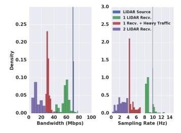
Fig. 2: Streaming LIDAR over WiFi using the Robot Operating System (ROS) produces high-bitrate point cloud streams, which can lead to a server receiving less than half the data (as pictured) or even network failure in the multi-robot setting.
