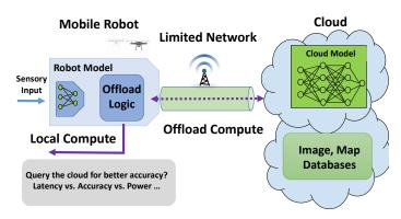
Fig. 1: Autonomous mobile robots are faced with a key tradeoff. Should they rely on local compute models, which could be fast, power-efficient, but less accurate? Or, should they offload computation to a more accurate model in the cloud, which increases latency due to congested networks? We propose a novel algorithmic framework to address such tradeoffs.
