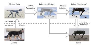
Fig. 2. The framework consists of three stages: motion retargeting, motion imitation, and domain adaptation. It receives as input motion data recorded from an animal, and outputs a control policy that enables a real robot to reproduce the motion.
