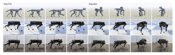
Fig. 1. Laikago robot performing locomotion skills learned by imitating motion data recorded from a real dog. **Top:** Motion capture data recorded from a dog. **Middle:** Simulated Laikago robot imitating reference motions. **Bottom:** Real Laikago robot imitating reference motions.
