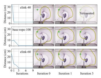
Fig. 7: Adaptation to robot embodiment. We varies the robot's last link with 3 different lengths (40,50,60cm), which effectively changes the mapping between the actions and their effects. As expected, the robot with a different link than training (elink-40/-60) has a higher initial error. However, for all variations, the system is able to reach the goal by adjusting its action according to the visual feedback.
