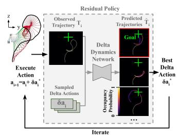
Fig. 3: Iterative Residual Policy. During each action execution, the tip trajectory is recorded as an image. For each sampled delta action  $\delta a$ , the Delta Dynamics Network predicts trajectories resulting from applying each delta action. The delta action that is predicted to minimize distance to the target is selected for execution during the next iteration.
