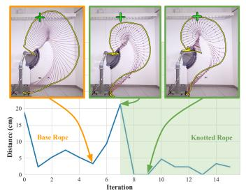
Fig. 9: **Online adaptation to system changes.** In this experiment, the robot first interacts with [base-rope-100]. At step 6, the rope is knotted. We plot the distance to goal with respect to the steps. While the tied knots significantly change the rope's length, density and mass distribution, the system is able to quickly adjust to the new system dynamics and achieve low errors.
