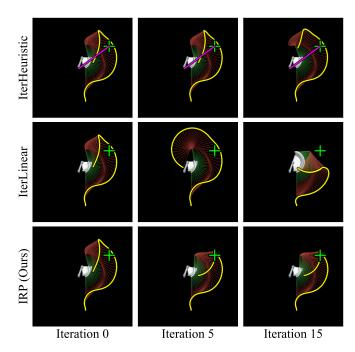
Fig. 8: **Comparison.** In this example, the rope trajectory switches between several discrete modes. As a result, IterHeuristic gets stuck in a sub-optimal orbit and iterLinear failed to approximate the switching behavior. In contrast, our method accurately predicts the switching behavior and reaches the goal.
