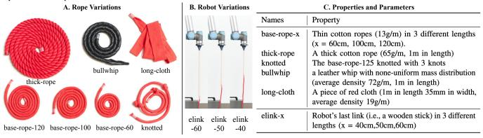
Fig. 5: **Real-world test cases.** A) Real-world testing ropes used to test our algorithm's generalization to untrained material, length, mass distribution and aerodynamics. B) By changing the the length of last link, the mapping from action parameters to effective swing speed and end-effector trajectory are changed simultaneously. C) Table for key properties and parameters for each real world test case.
