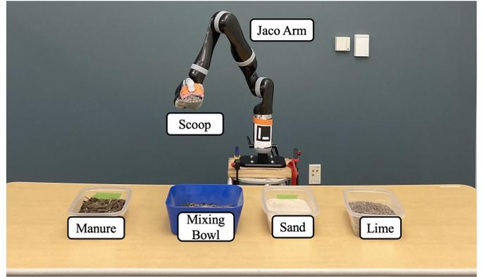
Fig. 1: Jaco robot setup: Subjects were required to teach the robot to create different types of soil mixtures in the mixing bowl using the sand, lime and manure available.
