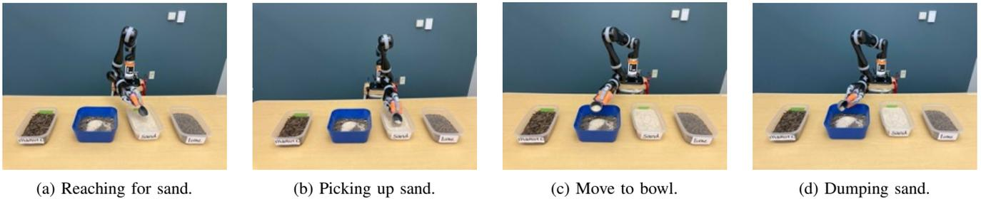
Fig. 3: Series of images demonstrating the plan created from learned trajectories on the robot to pick and drop sand from the set of 10 tasks created to test the learned policies from different demonstrations. For more details refer Appendix B.1.
