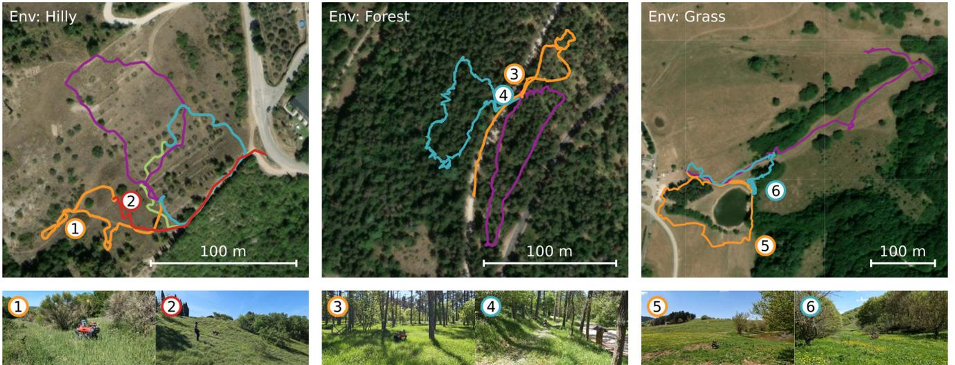
Fig. 12: Aerial views of the 3 environments used for offline testing of our system, illustrating the paths used for data collection and scene examples. The purple  $\blacksquare$  trajectories are used for training and the remaining for validation.
