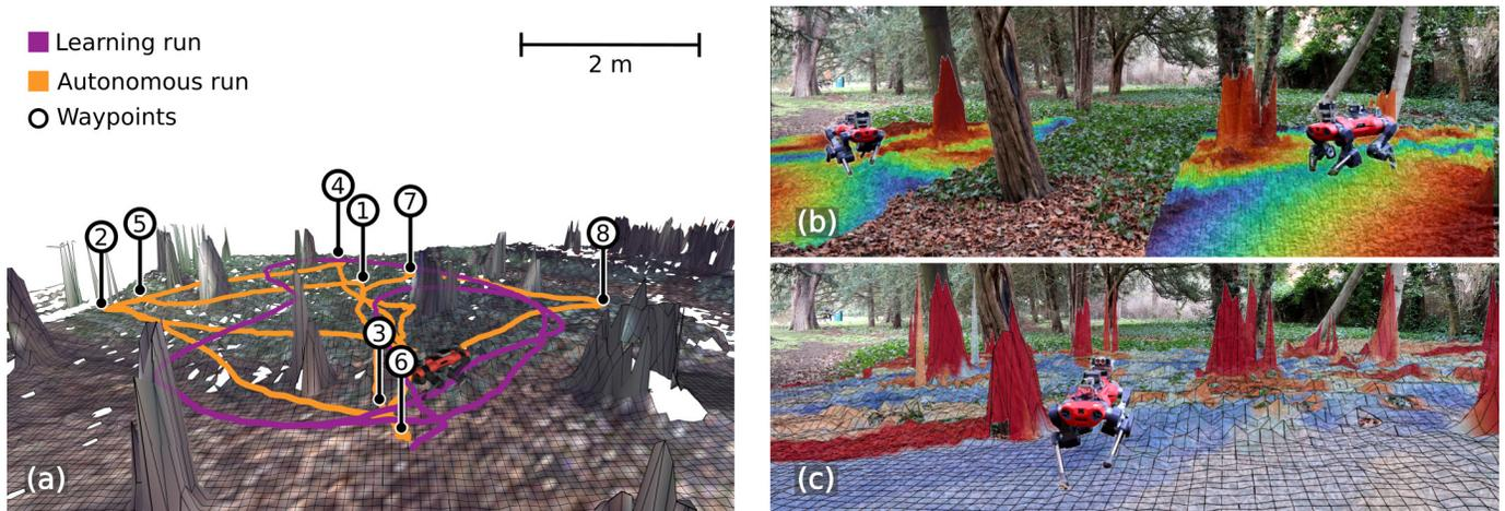
Fig. 10: Point-to-point autonomous navigation: (a) After teleoperating the robot for 2 min (path shown in  $\blacksquare$ ), we successfully achieved autonomous navigation in a woodland environment (path shown in  $\blacksquare$ ). (b) Some of the *SDF*s generated from the predicted traversability during autonomous operation. (c) Global 2.5D reconstruction of the testing area and predicted traversability, generated in post-processing to illustrate the capabilities of our approach.
