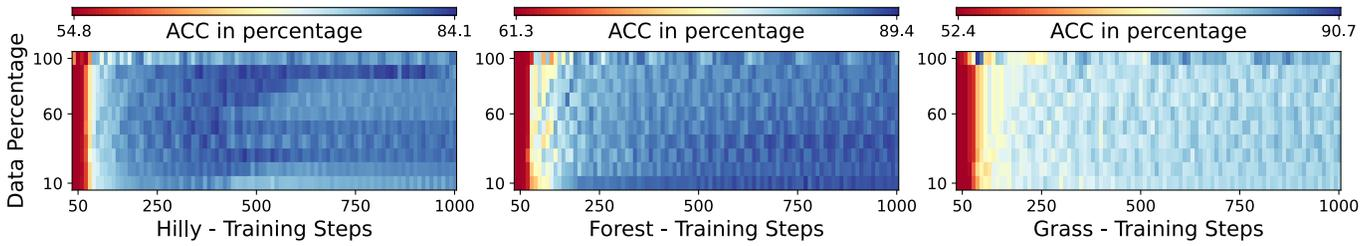
Fig. 13: Adaptation Speed vs Dataset Size: The performance measured by the accuracy increases over training as expected. In the limit case of training for a few steps ( $< 50$ ), the performance is equally degraded — independent of the dataset size. A small dataset size is sufficient for good performance. Please observe the different color scales for each environment. In the *Grass* environment the color scale is distorted by an outlier when using 100% of the data after 70 steps.
