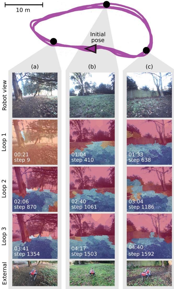
Fig. 8: Adaptation on real hardware: We tested the online adaptation capabilities of our system by teleoperating the robot to complete 3 loops in a park (top, route shown in  $\blacksquare$ ). The columns show different parts of the loop (a,b,c); each row displays the improvement of the traversability estimate over time and training steps.
