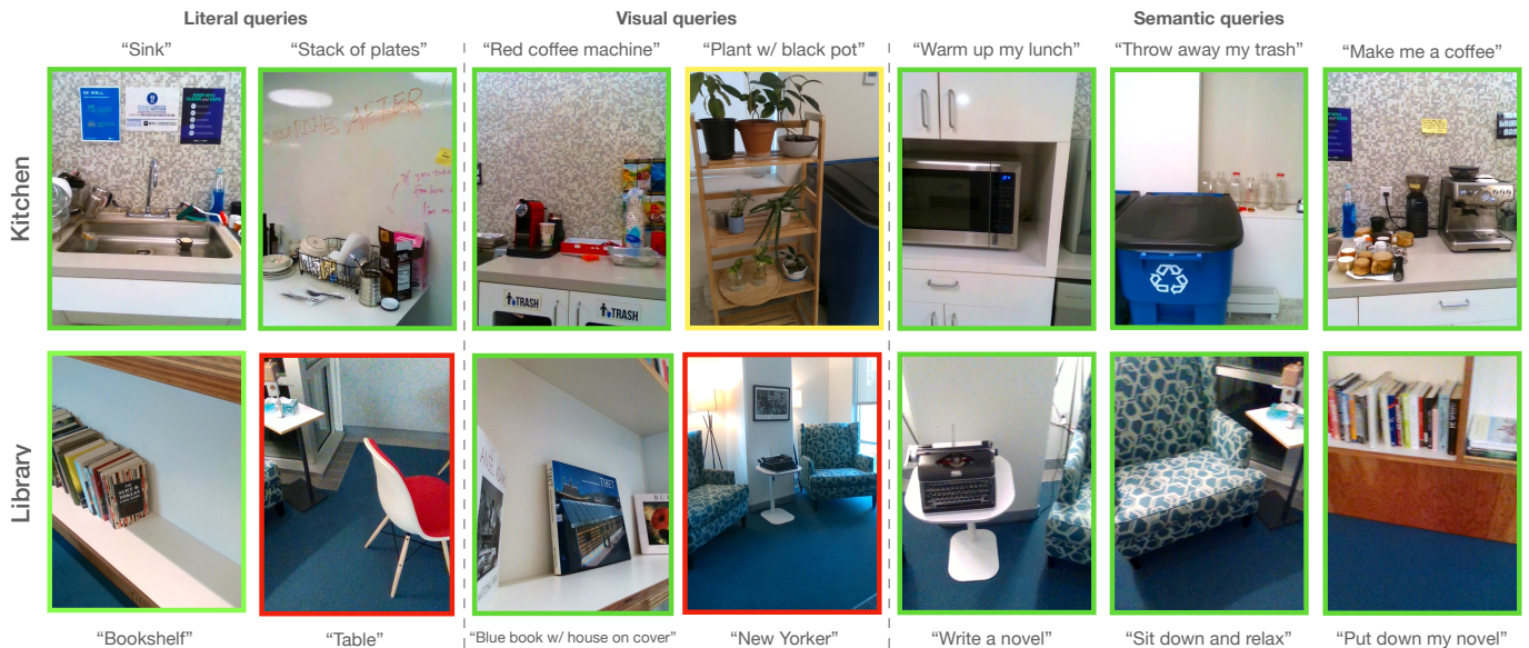
Fig. 10: Examples of the robot’s semantic navigation in two different testing environments, looking at objects given different queries. The images show the robot’s POV given the associated query, with color coded borders showing approximate correctness. The rows show different two different scenes, top being in a lab kitchen and the bottom in our lab’s library/lounge space, shown in detail in figure 9.
