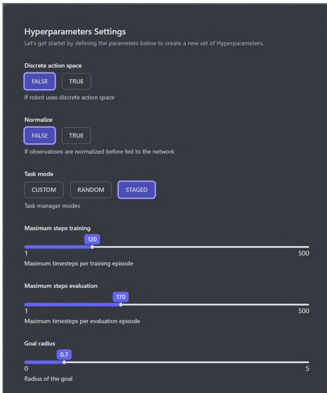
Fig. 6: Hyperparameter setting for the training tasks. The user can choose from a number parameters such as the task mode, training step size, evaluation step size, etc.
