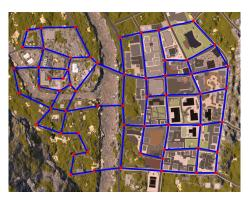
Fig. 1: Polypixel, a simulated urban environment used for our experiments (as seen in [7]), with its graph-based abstraction superimposed. Vertices show locations where a task has been assigned to one or more robots of a heterogeneous team. Edges represent travel paths between two locations.
