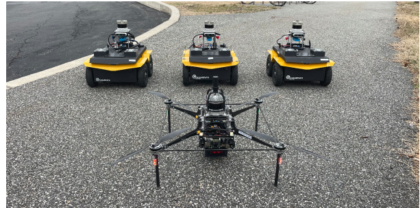
Figure 1: Robot platforms used in our experiments. Both platforms are capable of long-range GPS-denied autonomous navigation. In the experiments of this paper, the UAV relies only on cameras and the IMU for state estimation, while the UGVs rely on lidars. We refer readers to [1] and [2] for details on our UAV and UGV platforms.
