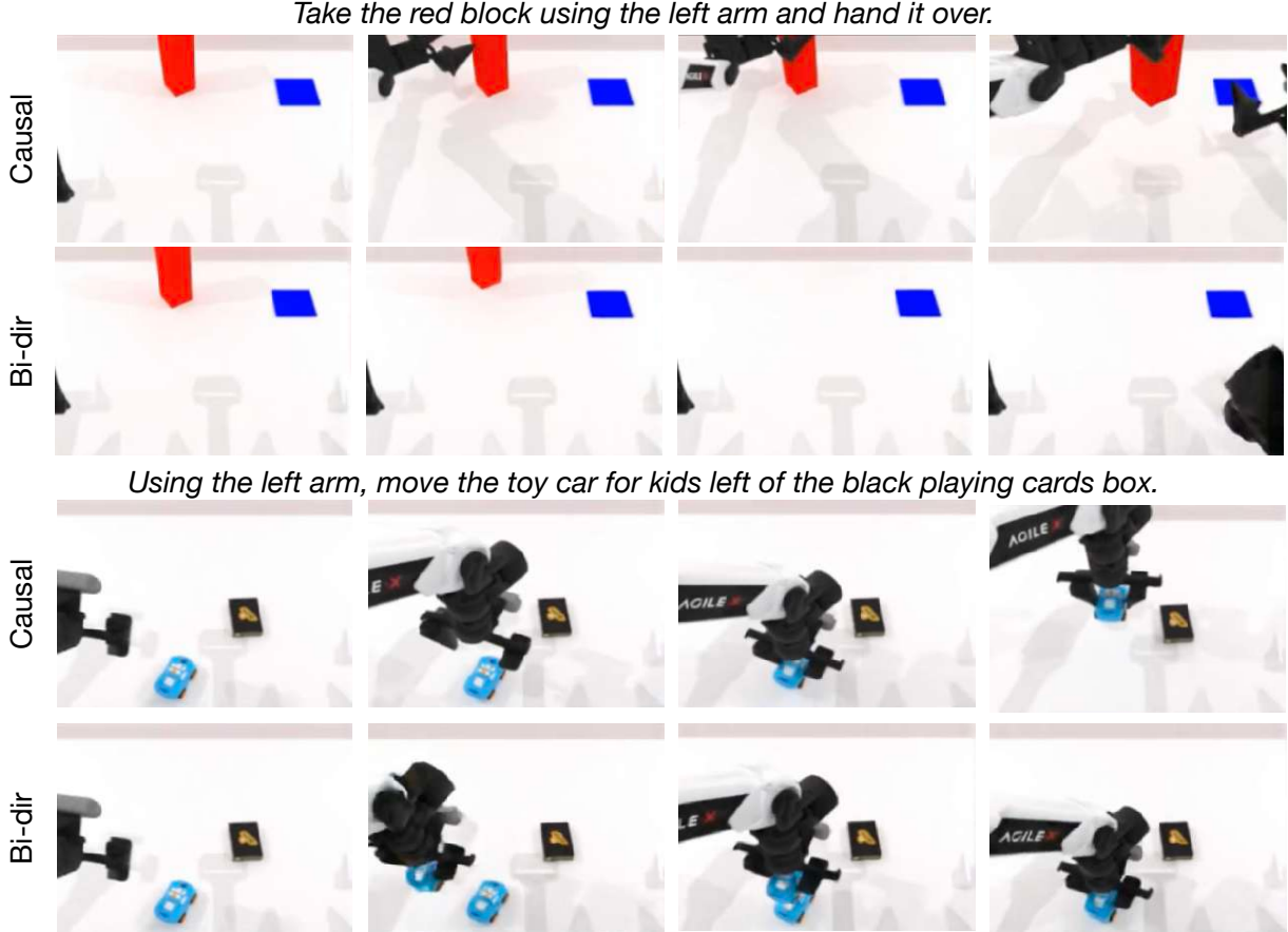
Fig. S1. Causal vs. bidirectional video quality. Bidirectional models produce videos with temporally inconsistent artifacts that violate physical causality, whereas our causal formulation generates videos respecting correct temporal logic.
