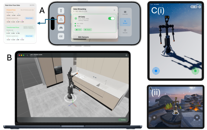
Fig. 6: Our iOS app ecosystem for multi-modal data streaming and sim-like interactive control.
