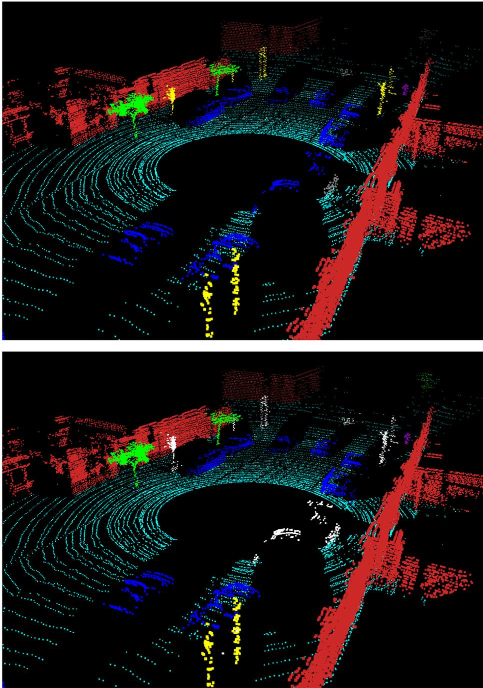
Fig. 6. (top) Ground truth classification for part of a 3D laser scan. Colors indicate ground plane (cyan) and object types (green: tree, blue: car, yellow: street sign, purple: person, red: building, grey: other, white: not classified). (bottom) Classification achieved by our approach. As can be seen, most of the objects are classified correctly. The street signs in the back and the car near the center are not labeled since they are not close enough to any exemplar.
