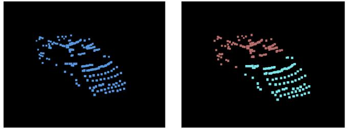
Fig. 2. (left) Laser points of a car extracted from a 3D scan. (right) Segmentation via mean-shift. The soup of segments additionally contains a merged version of these segments.
