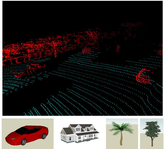
Fig. 1. (Upper row) Part of a 3D laser scan taken in an urban environment (ground plane points shown in cyan). The scan contains multiple cars, a person, and trees and buildings in the background. (lower row) Example models from Google’s 3D Warehouse.
